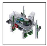
The main component of the R-CROP is a mobile robot that moves throughout the garden on a raised monorail track. This robot plants seeds using a special seed module with one compartment for seeds, and another for vermiculite.
